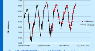
Fig.10: OCOG/Threshold SARin height comparison against Tabatinga gauge data. RMS 29.9 cm.
