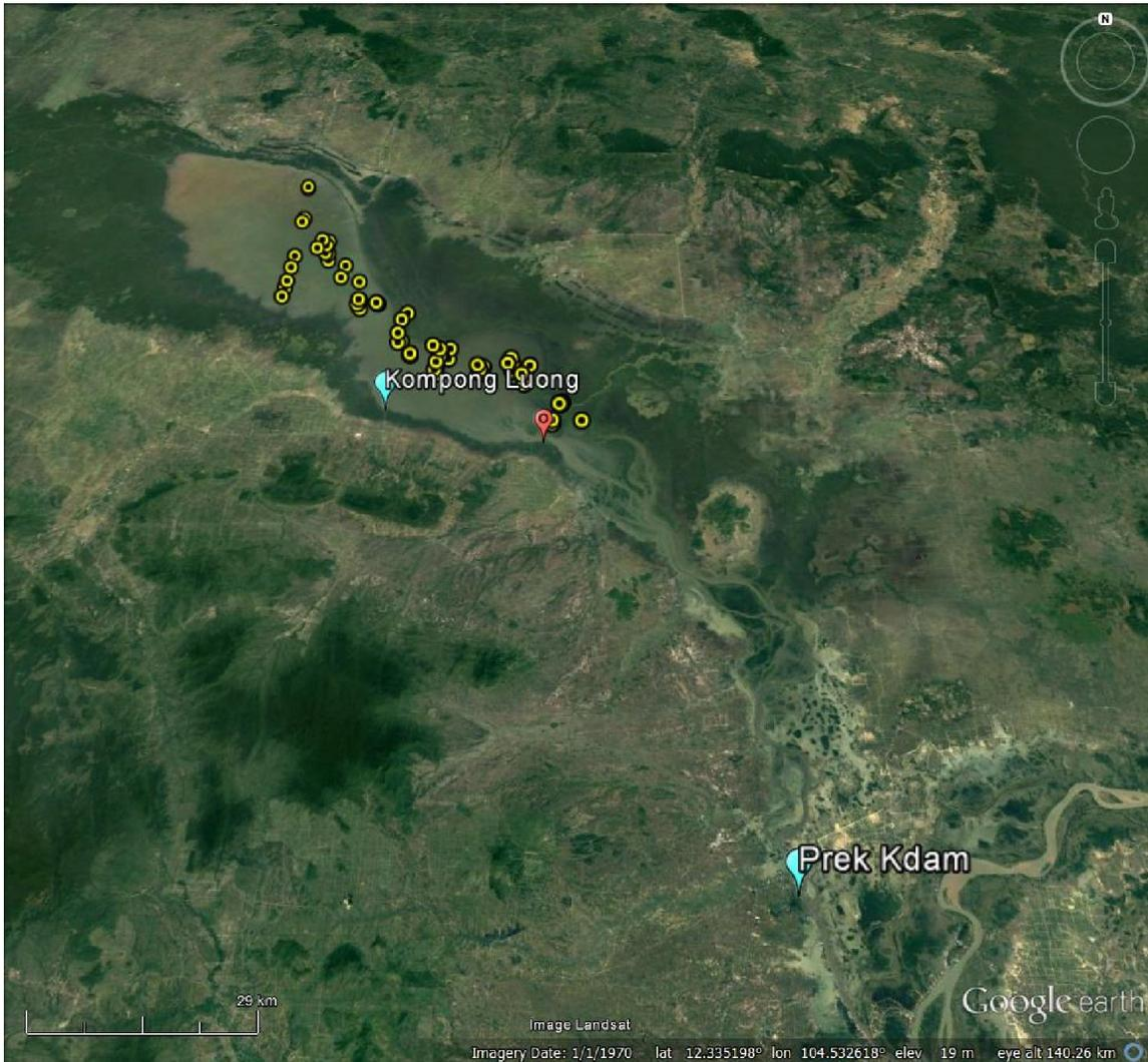
**Figure 6: Google earth image of Tonlé Sap. The locations of the 62 Cryosat-2 heights are given by the yellow circles. The location of the two gauges are indicated by turquoise markers. The position of the S-N OSTM altimetric pass is given by the red marker.**
