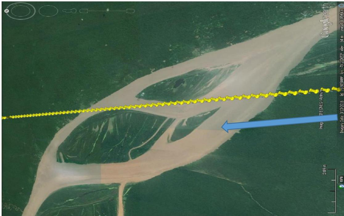
Figure 43: Google earth plot of ascending pass on 5 May 2012 across Amazon near Tabatinga (upper). Cross angles (deg) from SARin mode. The blue arrow points along direction of flight.
