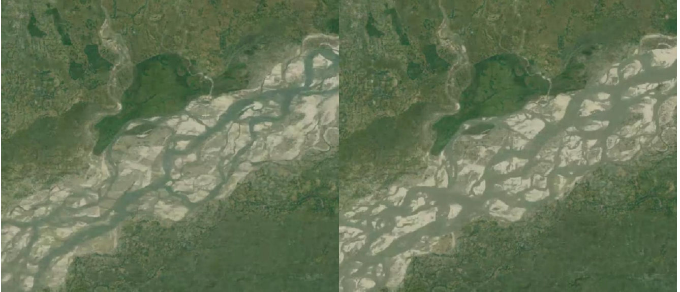
Figure 42: Landsat 7 images of the same part of the Brahmaputra river in the Assam valley showing the dynamic changes in river morphology. Left: 2010. Right: 2011.
