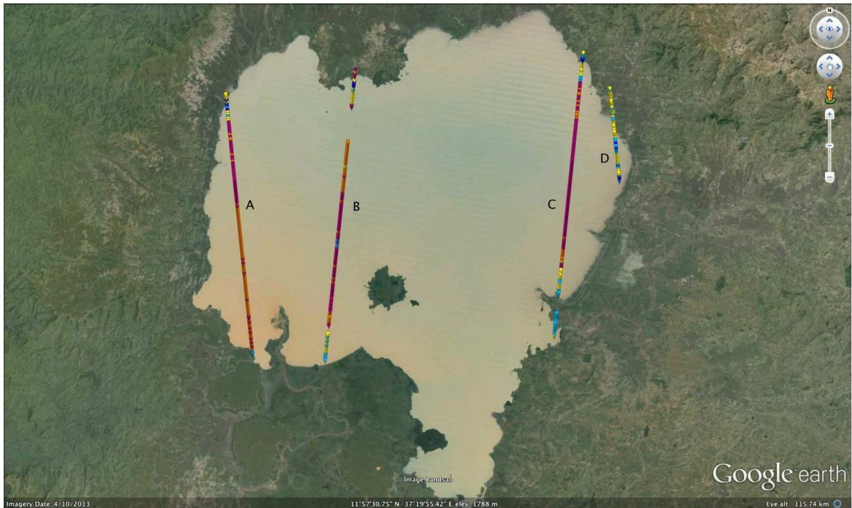
**Figure 4 Cryosat-2 tracks over Lake Tana (A is track number 4488, B track 3540, C track 4351, D track 3648)**
