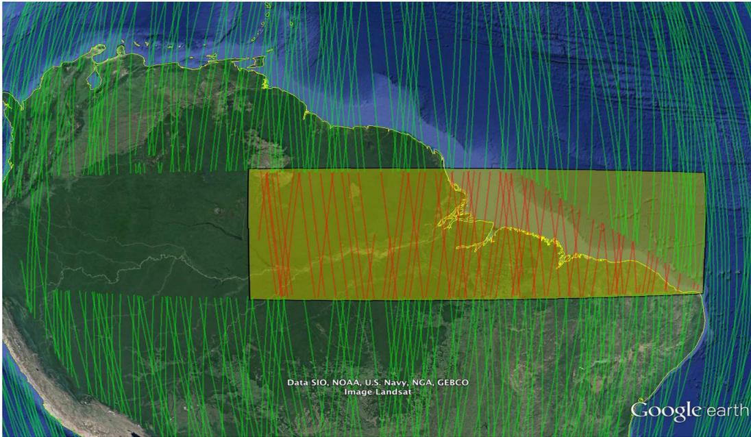
Figure 12 Amazon River Cryosat-2 tracks. Red shows the SAR tracks and green the LRM tracks
