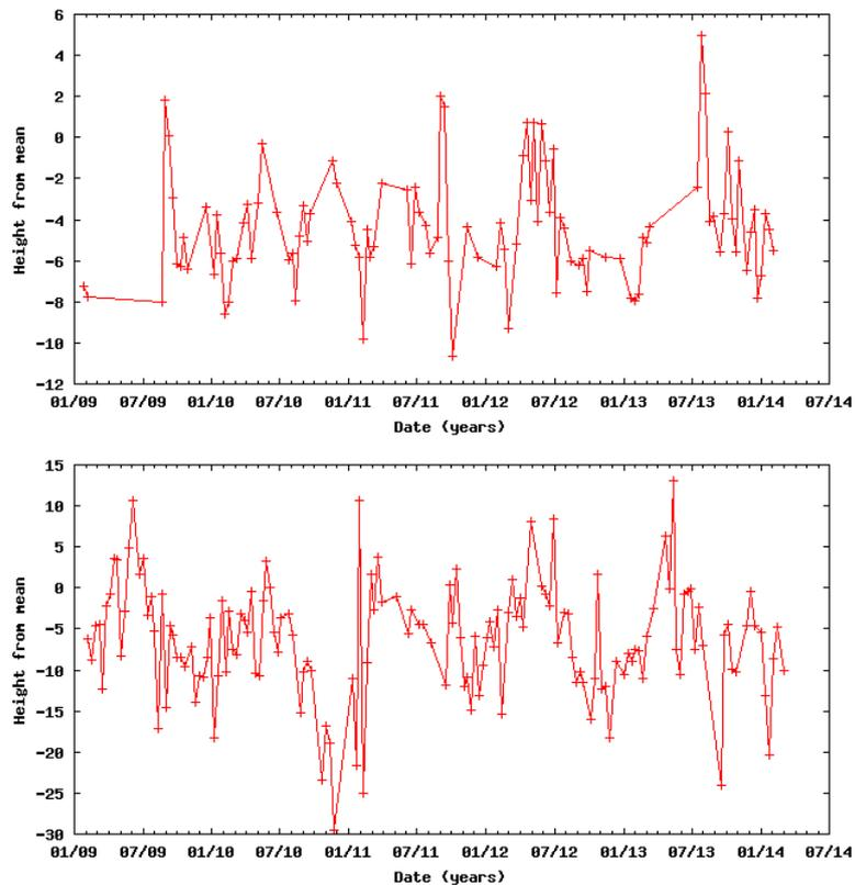
Figure 11 Jason-2 satellite altimetry data for the Amazon River from 2009-2014
