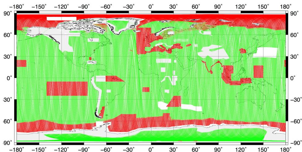
**Figure 1 Cryosat-2 tracks. Red are in SAR mode, Green in LRM mode and the blank areas SARIN mode.**
