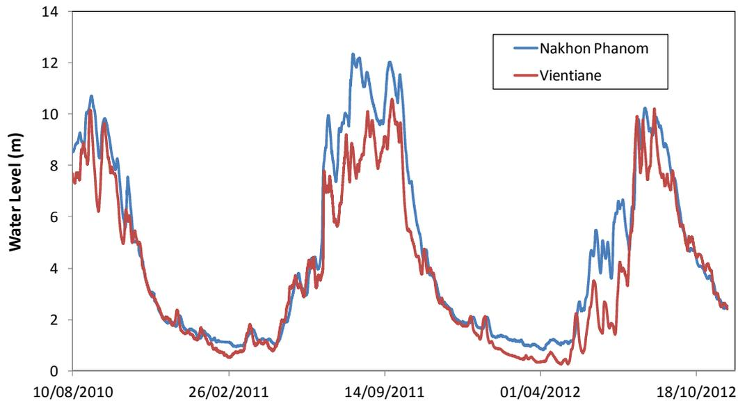
**Figure 16 Measured in-situ water level data for Nakhon Phanom and Vientiane on the Mekong river. The location of Nakhon Phanom and vientiane can be seen in Figure 15.**
