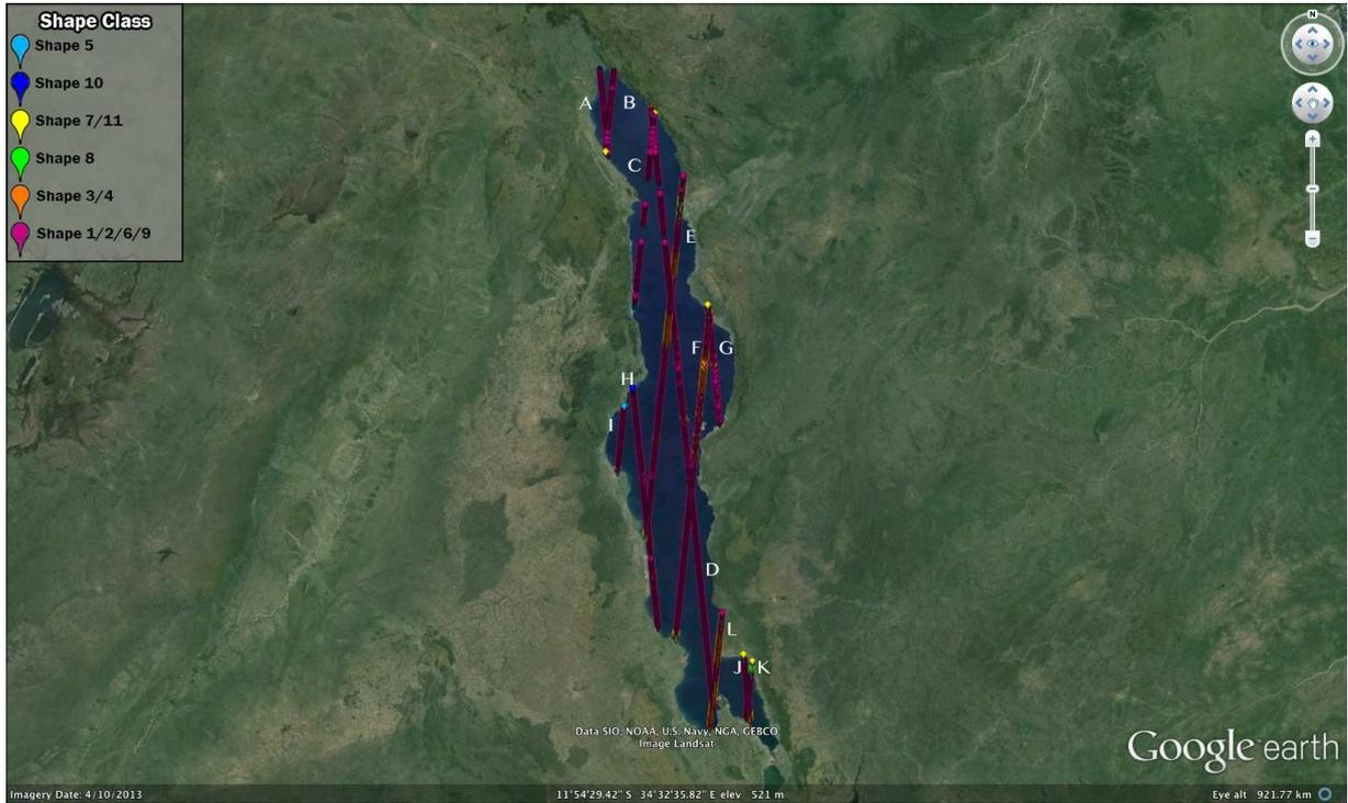
**Figure 8 Cryosat-2 tracks over Lake Malawi (11 tracks which correspond to letters A-K )**
